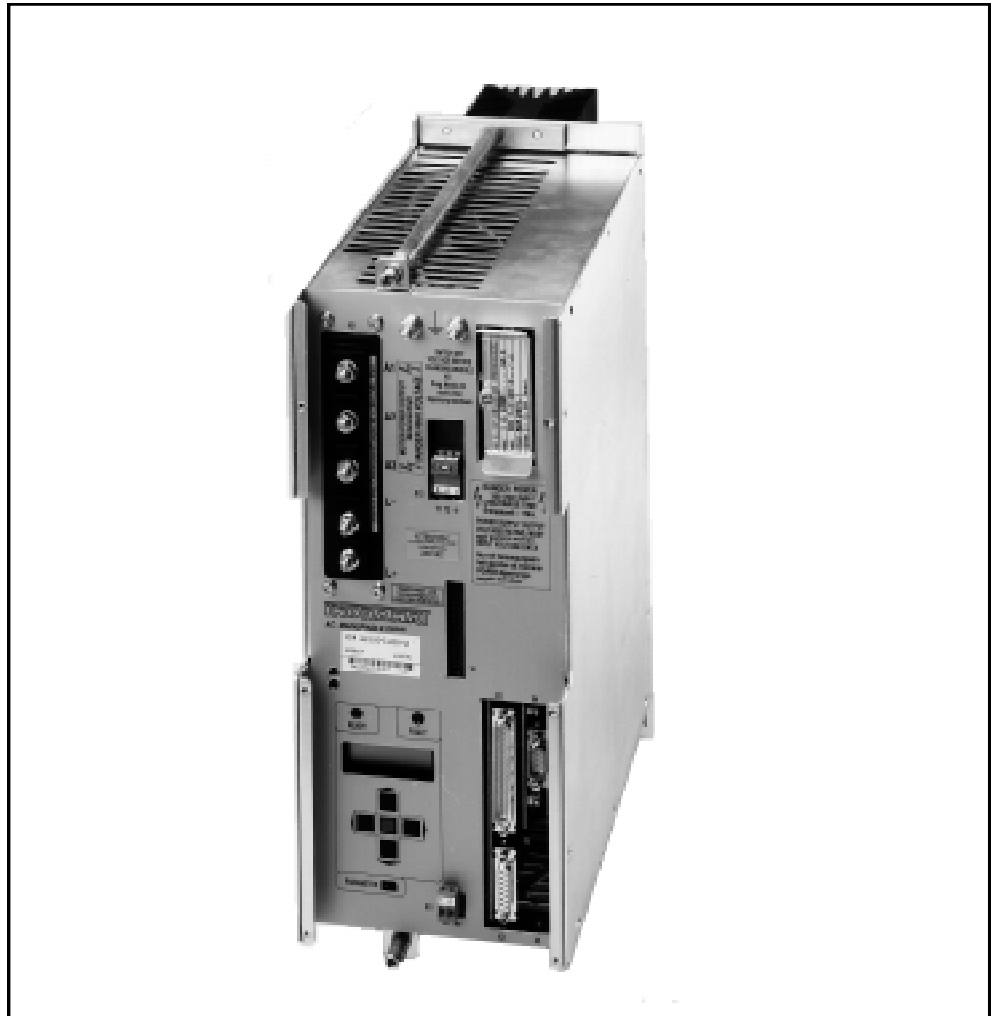
Fig 1.1 Modular KDA 3.2 Main Spindle Drive
